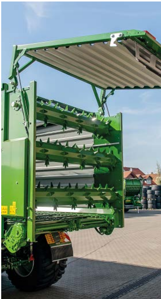
Wide opening, sturdy tailgate with mechanical locking – for fast unloading.
