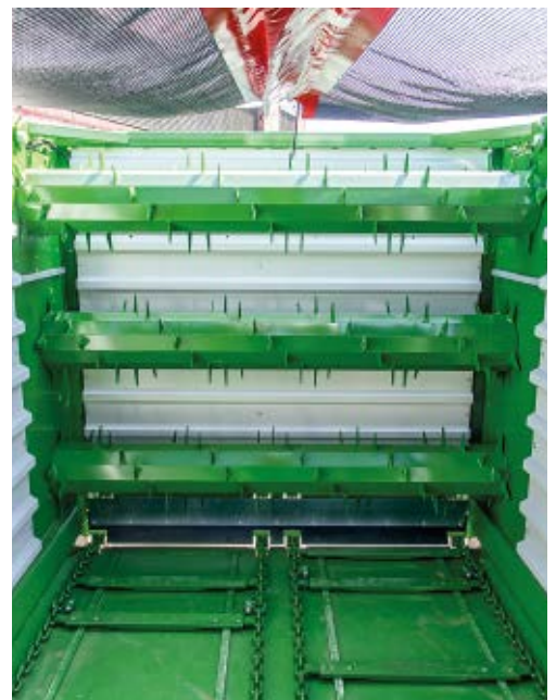
The S-model dosing unit with three standard dosing rollers ( CAREX 370 S / CAREX 410 S ).
